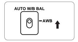
How to use the automatic tracking white (ATW) balance mode The automatic tracking white balance mode is established when the white balance selector switch (AUTO W/B BAL) is set to the ATW position. However, since the ambient light conditions may make the auto tracking white balance operation unstable, learn how to use the MEMO. PRESET and ATW modes to best suit the prevailing
